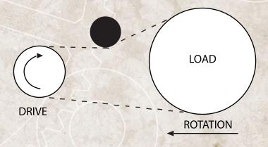
**Poor Sprocket Alignment** creates heat and may even bend the shafts on the drive system, causing great damage.
