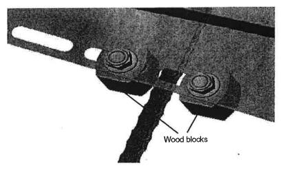
2. Install roller to uppermost portion of bottom slot. (chain should have a minimum deflection of 1/2 inch)
